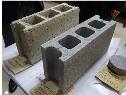
Figure 12 Comparison of CHB. Right: appropriate quality CHB. The shape and dimension are precise.
