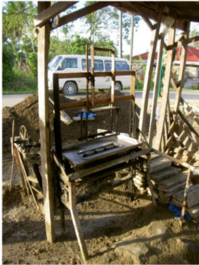
Figure 3 A small scale manufacturer of CHB. Left: simple manual manufacturing machine, Right: curing field for CHB in open air
