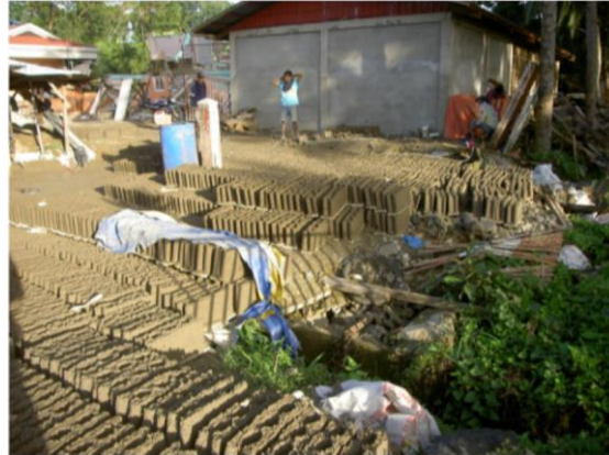
Figure 3 A small scale manufacturer of CHB. Left: simple manual manufacturing machine, Right: curing field for CHB in open air
