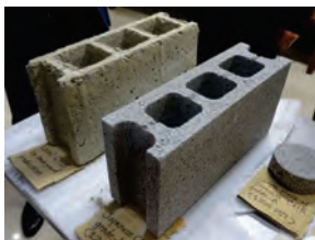
Both look similar in size and shape. The quality is very different. Left: Philippine made, Right: Japan made
